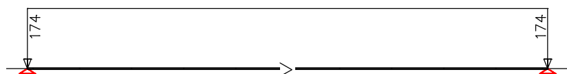
Load case 21: The dynamic coefficient Φ of 1.16 is already considered in the load ordinates.
