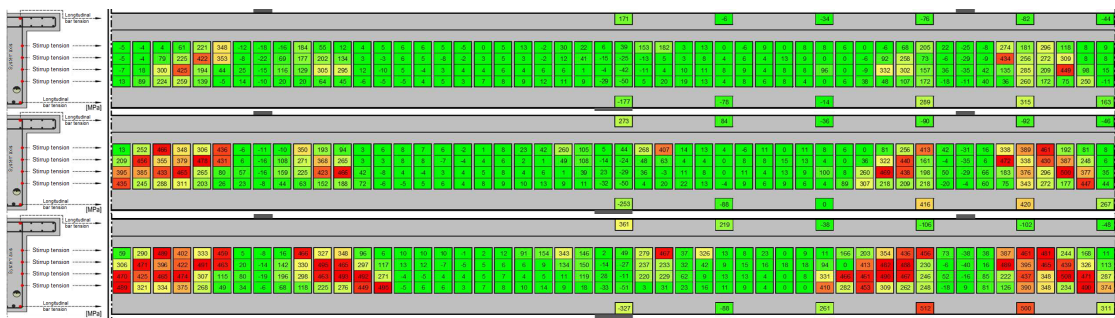
Measured stirrup stress \sigma [MN/m 2 ] at press forces of 1200 / 1400 / 1540 kN BAST Book B 150, A.2.2.1 (c), (d), (e)
